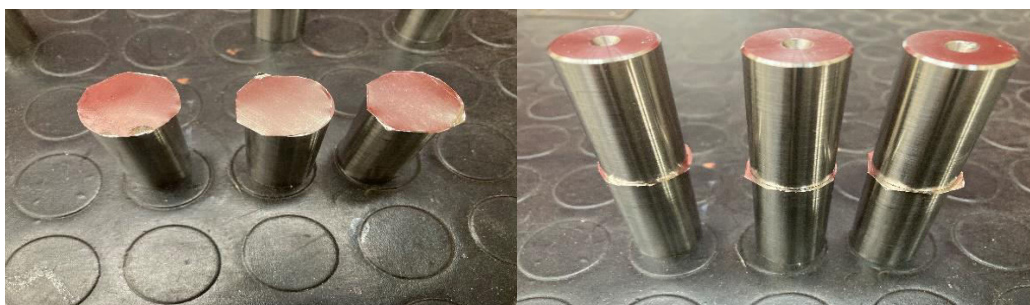
Fig. 4 Nickel foil shape and placement
