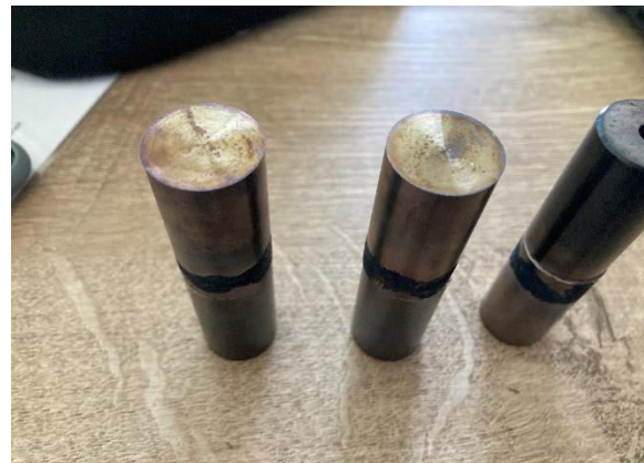
Fig.8 Brazing applied parts before machining.
