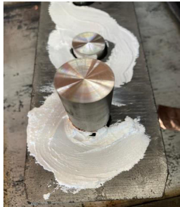
Fig.5 Application of Stop Off
